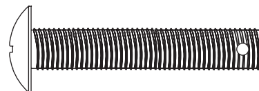
PHILLIPS TRUSS HEAD SCREW 1/4-20 X 1 1/2
