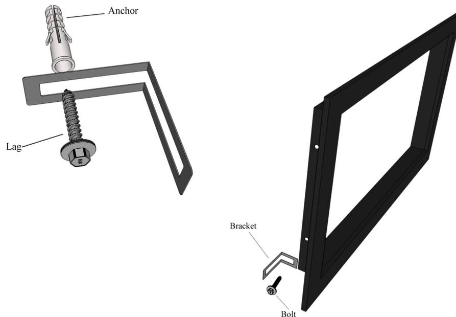
Once the frame is in the desired position, attach brackets to frame with bolts and nuts provided. You will want to bend the bracket in a manner that will allow it to make contact with the masonry firebrick inside the fireplace. It will also allow you to mark where you lead anchors need to be installed. The bracket needs to be flush to the firebrick surface so the lag will fully tighten to the anchor. Refer to the Ironhaus web-site installation instruction for illustrations.
