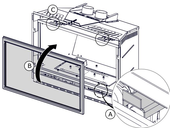
Re-install the door, ensuring to latch the two top latches.
