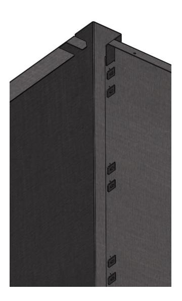
Note: Tabs have been laser cut in pairs. Repeated bending of the metal tabs will result in the tab breaking off. For this reason, only one tab out of each pair of tabs should be used. This will allow for any future addition or change to the kitchen as well as disassembly for the purpose of relocation.
