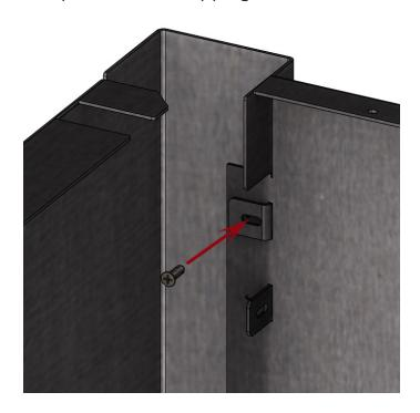
This process should be repeated until all vertical supports and front and back panels have been erected. While the order of construction can vary, it is recommended that all back panels be erected before installing the front panels.
