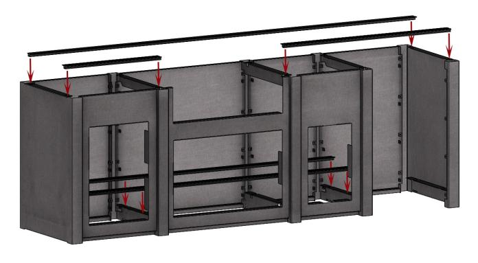
Where the horizontal rail intersects with a vertical support, install two (2) of the included self-tapping screws in the grooves on top of the horizontal rail.
