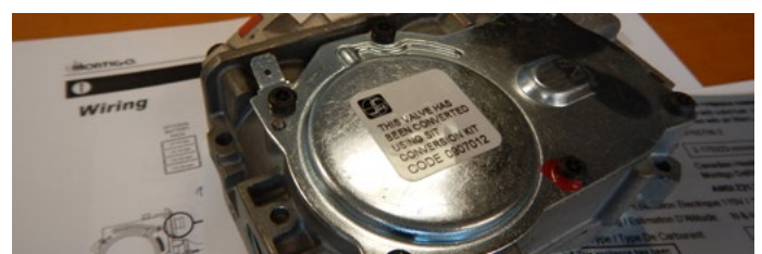
Figure 13.k Conversion label on valve
