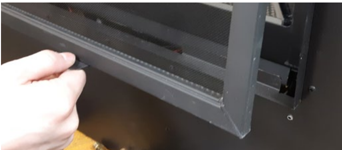
Figure 20.b Lift out the Retaining Tabs and screen
