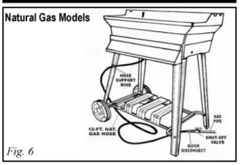
If the grill is to use Natural Gas from the supplied 12foot hose (Fig. 6): the hose must pass through the hose ring (See Fig. 1). The hose will have a quick-disconnect fitting at the source and the source will have a gas shut off valve with easy access.
