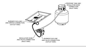
Test fire unit and check for leaks prior to full operation.
