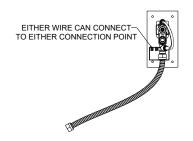
Carefully uncoil the thermocouple lead. Connect to the valve first by hand then tighten with a 10mm wrench. One thread should be visible when properly installed. **DO NOT** cross-thread thermocouple connection.
