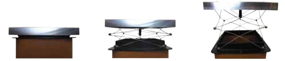
The Top Damper effectively seals in "paid" energy dollars. It mounts to the chimney top and seals with a flat rubber gasket when closed. The Top Damper is constructed of premium stainless steel and cast-aluminum and won't rust like conventional cast-iron dampers. The control mounts in the firebox for quick and easy access and defaults to the open position.
