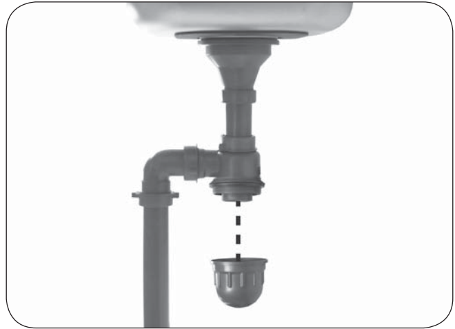
Fig. 4-1 Drain trap cleaning
