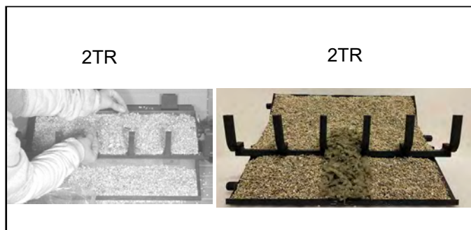
Figure 7.7 Rock Wool Placement
