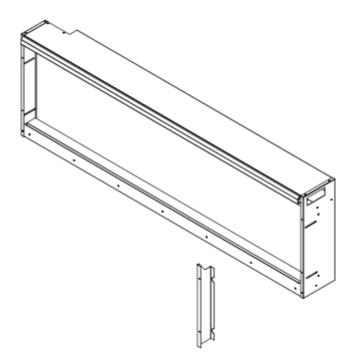
4. Put the trim back onto the appliance and fasten with screws.(NOTE: This step is to make sure that the fireplace fits the wall opening well and there is no gap between the trim and the wall after installation)
