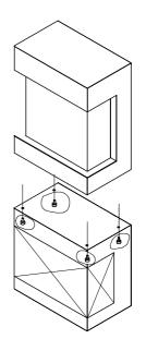
4. Plug into the back of the unit. Re-install the back steel panel.
