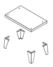
2. Unscrew the adjustable feet from the bottom of the unit.
