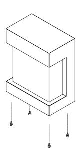
2. Unscrew the rear screws and remove the back steel panel
