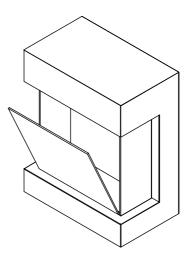
STEP 4: After finishing decoration, re-install the front glass panel using the securing screws removed in step 2.
