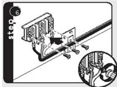
7. Reattach the Strain Relief Bracket
