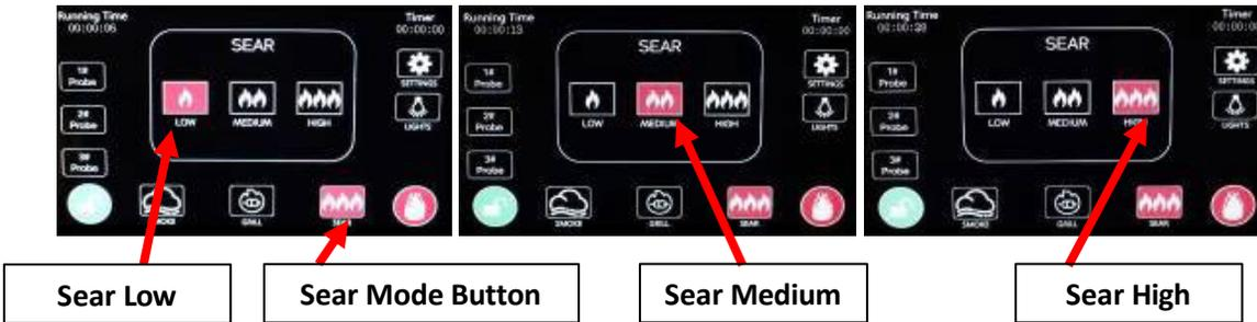
**IMPORTANT:** Only use the sear grate while the grill is in sear mode. Using the sear grate in smoke or grill mode will cause the grill to overheat.
