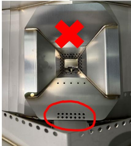
**Lip of the burner pot is above the pellet chute. Gap between the igniter and the burner pot.**
