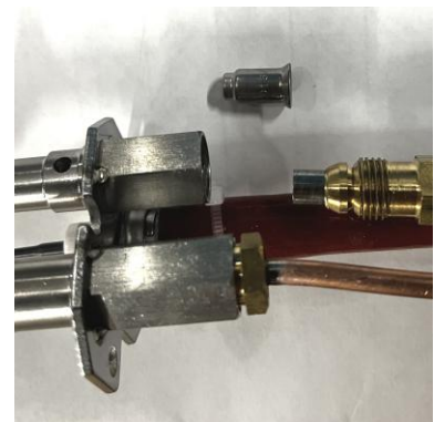
Figure 9.3 – Cleaning pilot orifice
