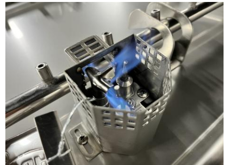
Figure 9.2 – Pilot flame coverage of thermocouple.
