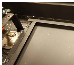
Figure 12.f Unscrewing brackets securing metal plate
