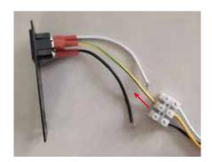
2. Attach the wiring to the junction block. Please make sure the live wire goes into the "L", the neutral wire into "N" and the ground wire into "G".
