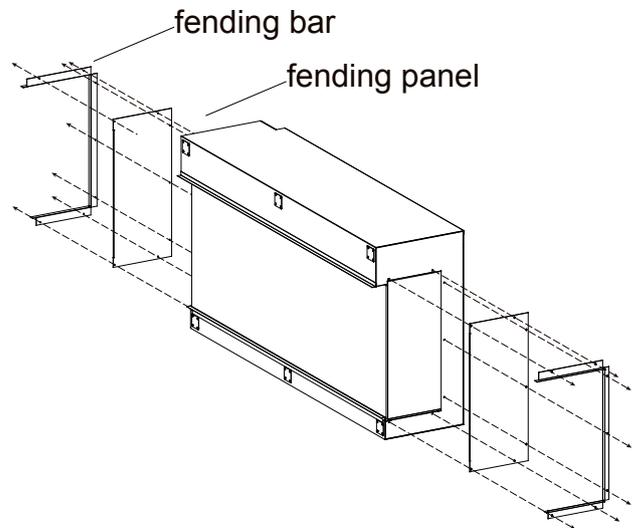
(2). Remove the fending panel on the left side if you want to view the flame from front and left side.
