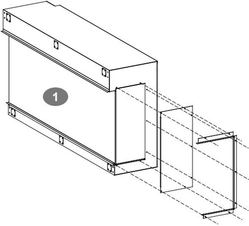
4. Unscrew 2 screws and remove the brackets which are fending the right side glass.
