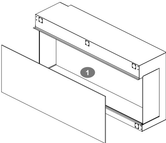
6. Remove the front glass, left side fending bar, fending panel, left glass and brackets from the other one in the same way.
