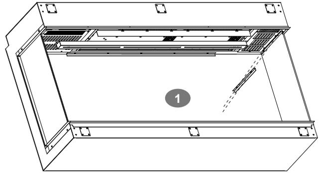
2. Unscrew 3 screws (The quantity varies depending on the size of the unit) and remove the front glass bracket which are fending the front glass.
