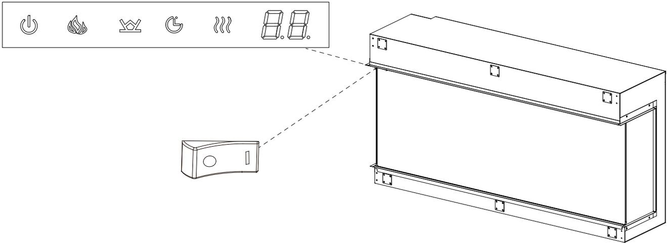
Touch the control panel once to “wakes up” the controls. This will cause the controls to light up. At this time, you can press the power button to turn on fireplace
