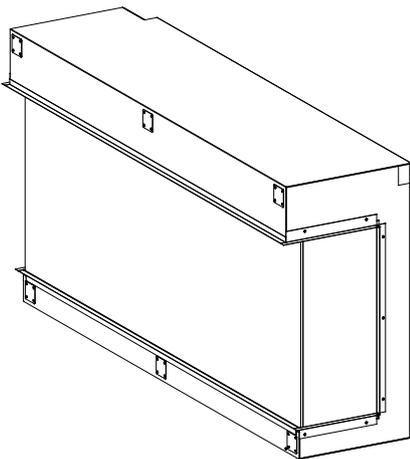
4. Remove the framing plates from the fireplace and save for step 6.
