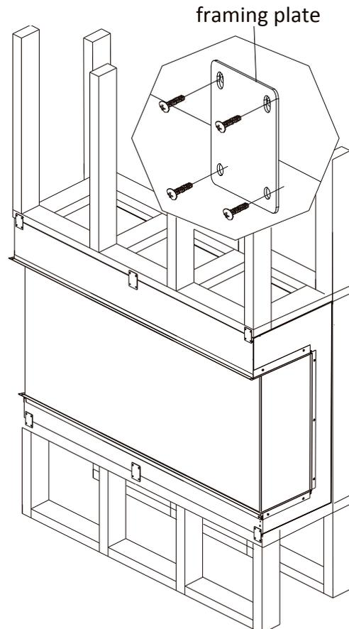
7. After checking that the fireplace operates properly, cover the glass panels with protective plastic bag and install plywood or drywall.
