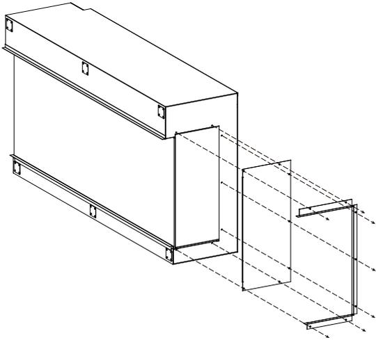
3. Screw back the fending bar after the panel is removed.
