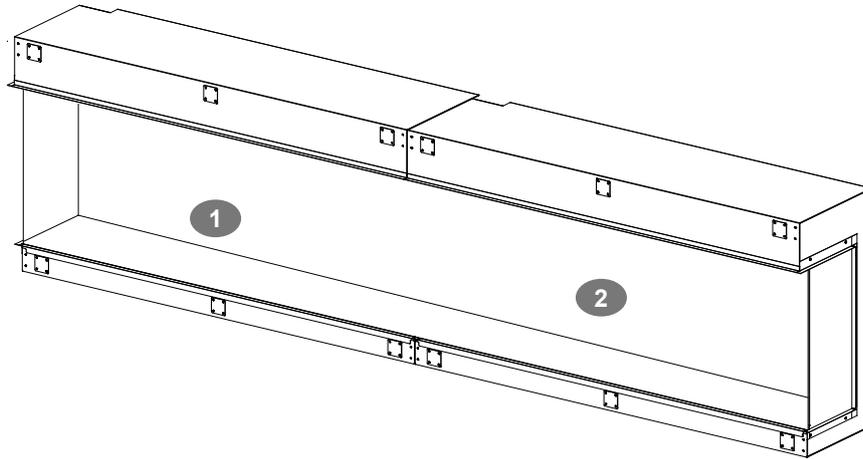
8. Unscrew the 8 screws at the joint, then remove the 2 framing plates from the fireplace 1 and fix them as the picture shows.
