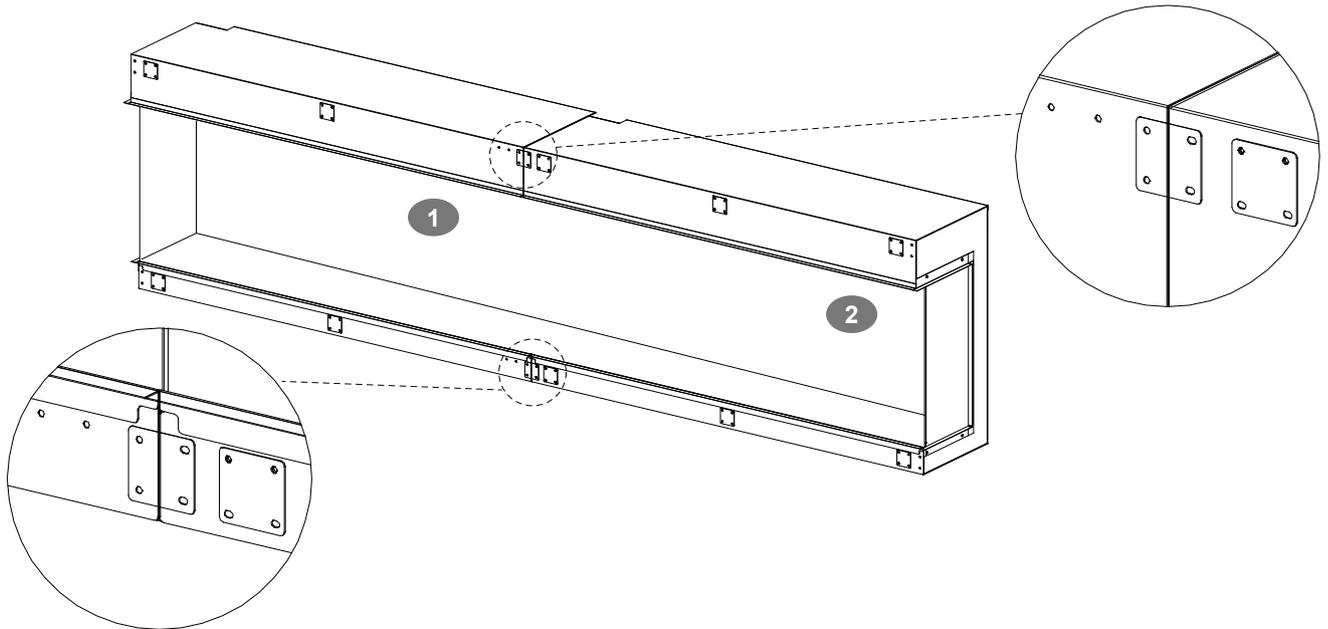
9. Put back the front glass to the fireplaces and secure them with screws and front glass brackets.
