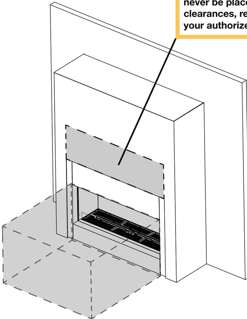
**Fireplaces generate radiant heat. Do not put objects in front of the appliance (minimum distance of 4 feet [1.12m]).**
