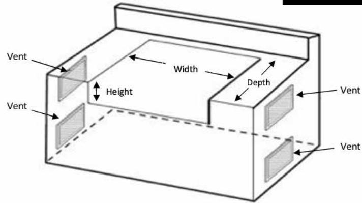
Minimum of 2 vents, but optimally 4 vents, per cabinet that has any sort of gas supply or connection. Each vent must be at least 20 sq inch in size and have access to outside/fresh air.
