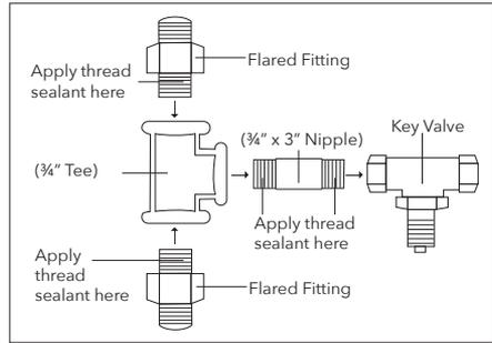
**7. CONNECT FLEX LINES TO COUPLING AND KEY VALVE CONNECTION**
