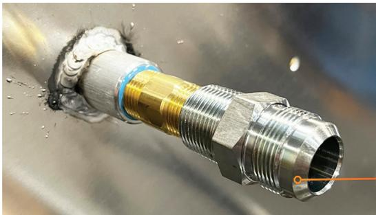
Photo 17: Attaching the Male Flare Hose Adapter
