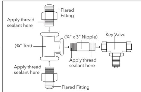
**6. CONNECT FLEX LINES TO COUPLING AND KEY VALVE CONNECTION**
