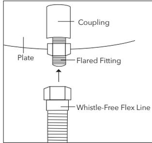
**5. LOCATE 2ND FLARED FITTING AND CONNECT TO KEY VALVE**
