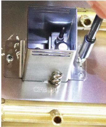
Photo 5: Securing the Pilot to the Plate/Pan
