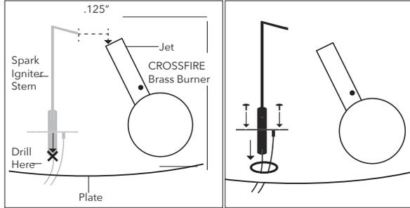
If the distance to the jet is greater than .125", you can adjust the position by **gently** bending the spark igniter by the stem. Bending too far can result in breakage. Do not flex at the existing bend, this can result in breakage. If the spark igniter is too far away or too close to the jet, you will not get a strong enough spark to light the burner.
