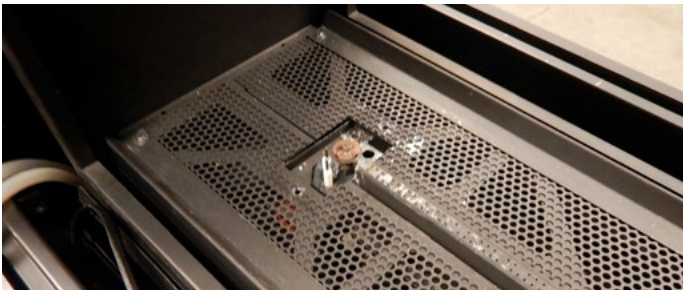
Figure 12. Removal of the pilot cover
