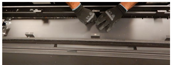
Figure 12.g Removing metal plate
